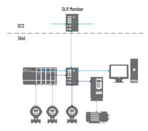
DLR MCC - Simplex Connected to DLR Ring
