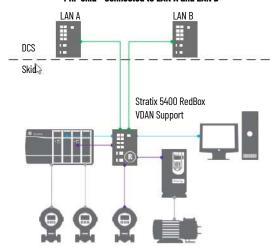
PRP MCC - Connected to LAN A and LAN B with DLR Ring
