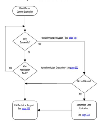
Figure 27 - Resolve Server to Client Communication
