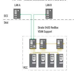
PRP Skid - Connected to LAN A and LAN B
