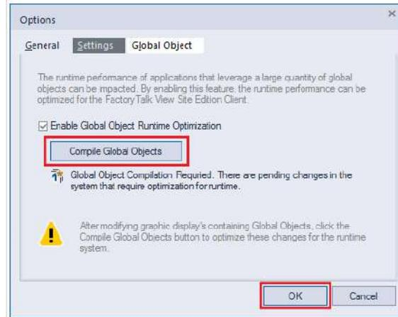
The first time that you compile global objects, the process can take an extended amount of time, depending on the number of displays in the application. Subsequent compiles require less time as they only process changes to displays.
