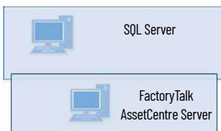
FactoryTalk AssetCentre software manages the information that is produced by each of its assets and processes the data into a SQL server. When performing a backup of FactoryTalk AssetCentre software, nothing must be done within FactoryTalk AssetCentre. To back up the FactoryTalk AssetCentre configuration and data, back up the FactoryTalk AssetCentre database in your SQL server.
